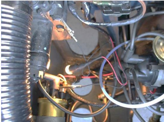
Static timing light with bulb connected
